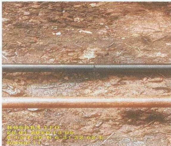
FIG. 1, Picture showing hacksaw cut.
